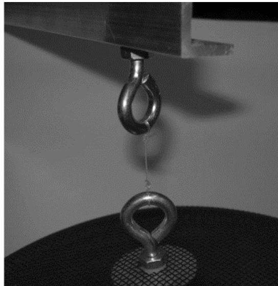
Figure 2. A photo of the 1.7 cm x 0.7 mm nylon filament used in the pendulum experiments.
